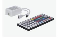
Basic RGB strips driver with radio remote control. Intuitive operation and smooth adjustment of light intensity.
