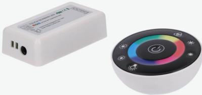
Driver for RGB strips with round radio touch remote control in black color. It allows you to control color and brightness.
