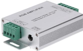
Power amplifier for drivers used when the driver power is not sufficient. Simple connection by using screw clamps.
