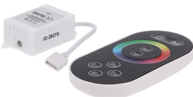
Driver for RGB strips with radio remote control in black color. Color and brightness control. Small dimensions of the driver.
